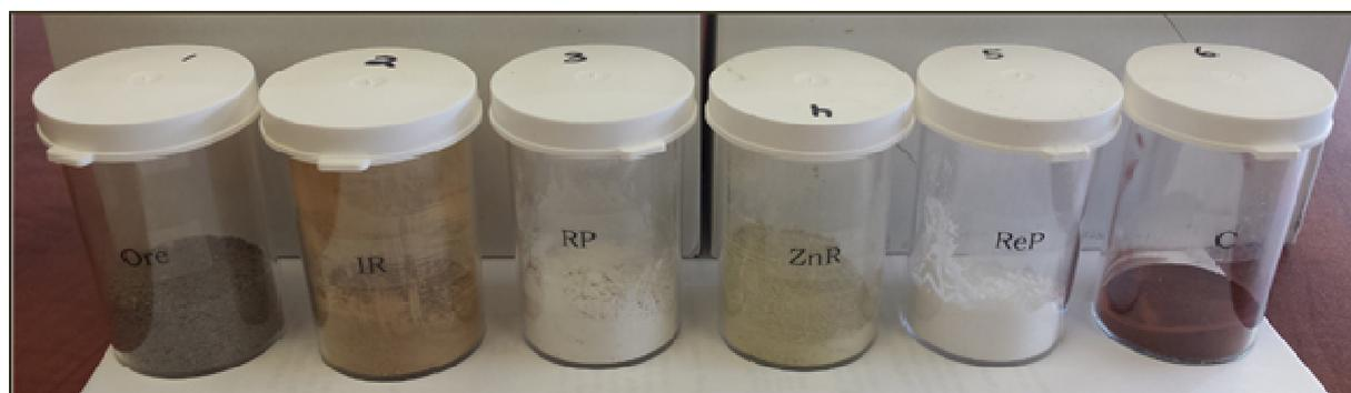
The process starts with finely crushed ore (vial 1 on the far left). The ore is then treated with acid, heated to 180<sup>o</sup> C and then water leached. The pH is then raised to precipitate iron to give an orangey stained residue (as seen in vial 2). This is the major solid product from the process and it is 'dry stackable' to give a stable, compact residue impoundment.
