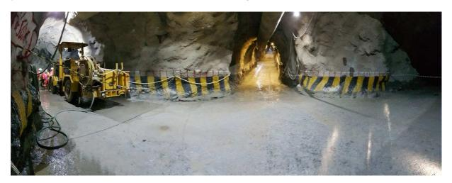
The ore drives are located along the footwall contact of the orebody. These footwall and ore drives extend to the limits of the orebody. Connections between the footwall and ore drives are developed as and when required.
