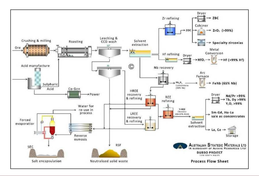
The crushed ore is then dry ground to the optimum particle size for good extraction of valuable elements. The dry ground ore is then mixed with concentrated sulphuric acid and roasted to form sulphated solids.
