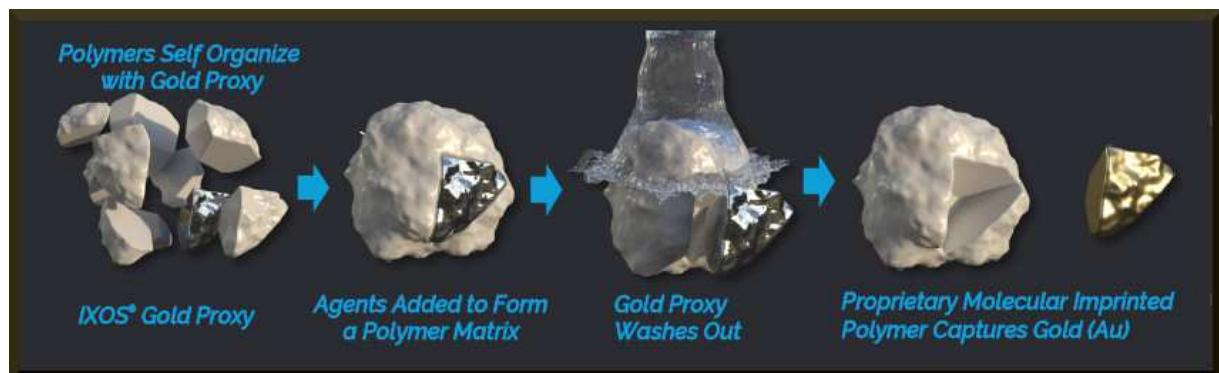
Below is another representation of the process. In some ways this strikes us as being the chemical equivalent of the Lost Wax Process used in casting:
