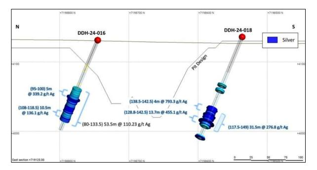
The team were particularly excited by the two holes shown above which are at an angle to the main trend of mineralization in the JAC southwest area and show broad mineralized intercepts including high-grade silver following a structural trend extending northwards towards Alpaca. The section is interpreted as showing the potential to expand the conceptual open pit and increase the JAC Mineral Resource and Reserve.
