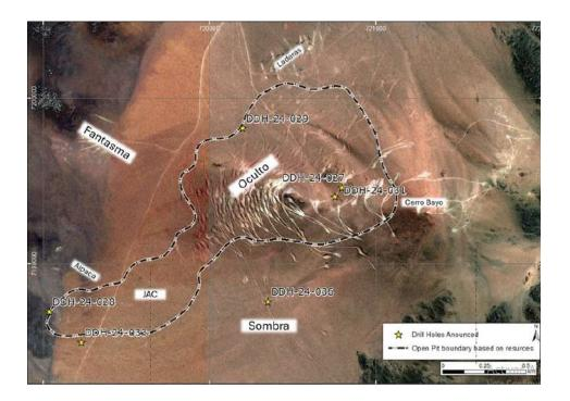
Hole DDH 24-036 was the first reconnaissance hole targeting this zone. Drilling intersected mineralization near-surface, with 22 m at 40 g/t Ag starting at a downhole depth of only 42.5m marking what the technical team regarded as a successful initial test of this new exploration area.
