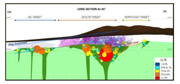
The sulphide mineralisation below the Oculto/JAC zones has only been sporadically drilled but the crosssection above was created to show the intercepts and a theoretical model, along the lines that Sillitoe suggested, showing the feeders for the higher precious metal's deposits, with the copper lower down in the structure, at very interesting grades.
