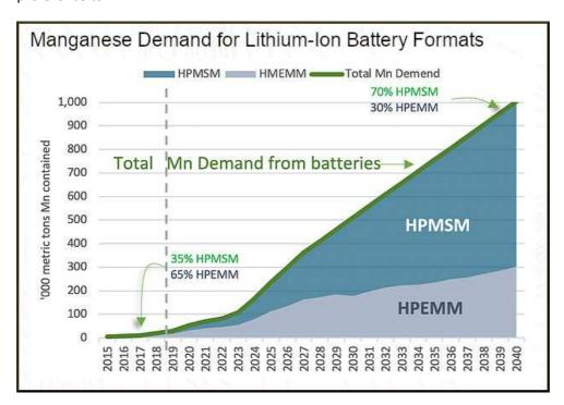
The forecast demand for Manganese in NMC and LNMO battery formats is weighted towards HPMSM in preference to HPEMM.
