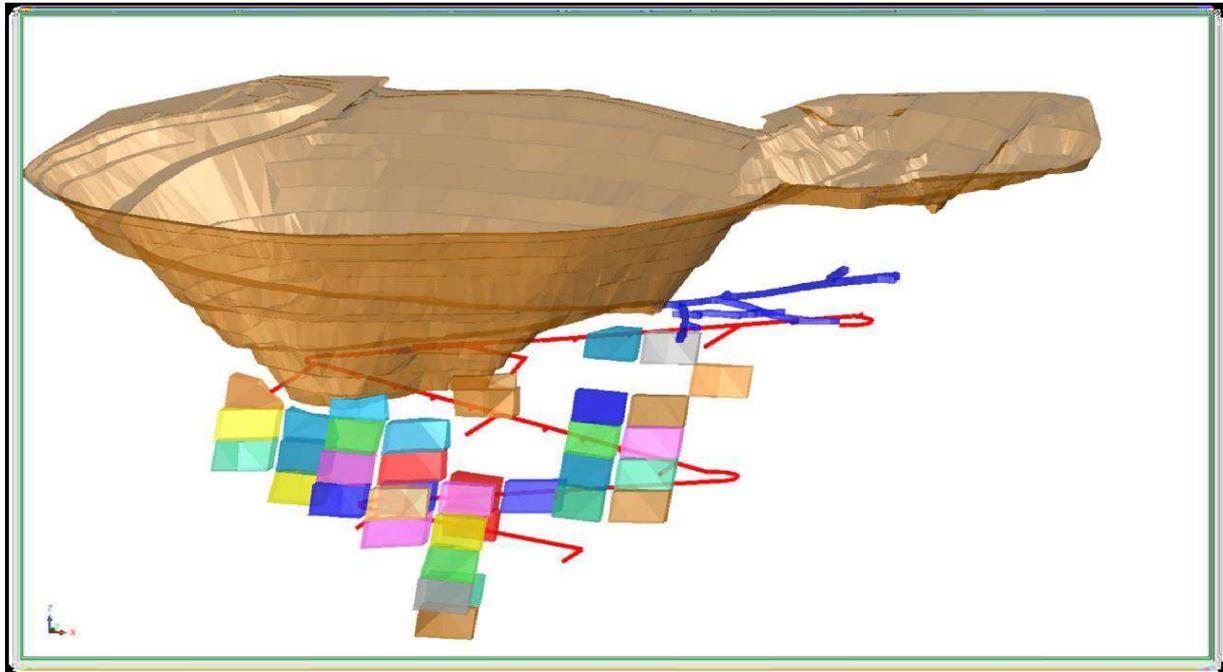
As of mid-2014 the decline (shown in dark blue below) from the Tau pit has been advancing towards a point underneath the Tawana pit. As part of the underground mine plan for Tau, the company will put in a vent through the floor of the Tawana pit. This will be done by expanding the current open pit at Tawana, which will provide additional ore for the processing plant in 2014. The company has mined 2,300 in situ oz to date with a further 4,000 oz targeted.
