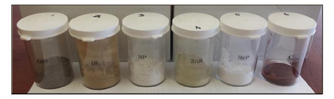
The process starts with finely crushed ore (vial 1 on the far left). The ore is then treated with acid, heated to  $180^{\circ}$  C and then water leached. The pH is then raised to precipitate iron to give an orangey stained residue (as seen in vial 2). This is the major solid product from the process and it is 'dry stackable' to give a stable, compact residue impoundment.
