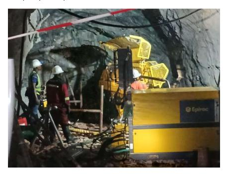
The mining method is long-hole open stoping (LHOS). As practiced here, the method involves holes being drilled from the level above into the void already opened below and then it is blasted collapsing the ceiling into the void where it is scooped up and transferred to surface.
